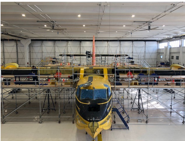
Pictured above: One of the specially selected CL-215 aerial firefighters undergoing upgrade and modification to CL-415EAF "Enhanced Aerial Firefighter" configuration at Longview's facility in Calgary, Alberta utilizing Viking-supplied conversion kits.
